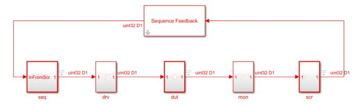
This feature allows you to tune sequence generation and control simulation according to run-time criteria calculated in the scoreboard.
